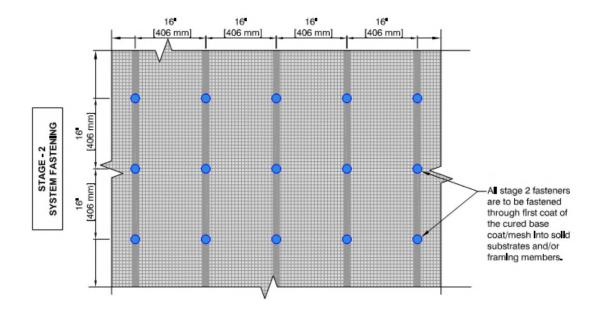
SPEC NOTE: The above fastening pattern addresses recommended fastener placement for typical wall installations. Consult Durabond Building Products Ltd. for project-specific installations.
